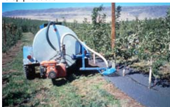
Prototype applicator for sprayable paper mulch in orchards, developed by Dr. Gene Hogue. Using reject fiber from paper recycling.
